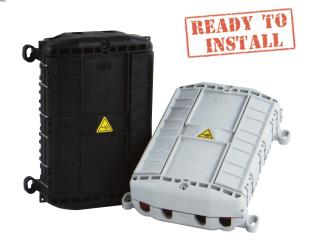
The highly versatile Focus-micrODC closure has been designed for the FTTH network and thanks to its peculiar features comply the new market requirements: compact dimensions (≤ 2 litres) mechanical (IK10) and waterproof protection (IP68); versatile and flexible usage (manhole, direct buried, aerial, facade installation) in outdoor environment. It is mechanically sealed and can be optionally provided with a pressure valve.
