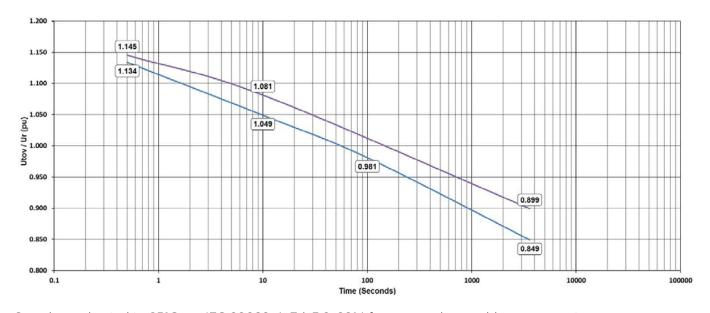
Samples preheated to 85°C per IEC 60099-4; Ed. 3.0, 2014 for screened separable surge arresters.
