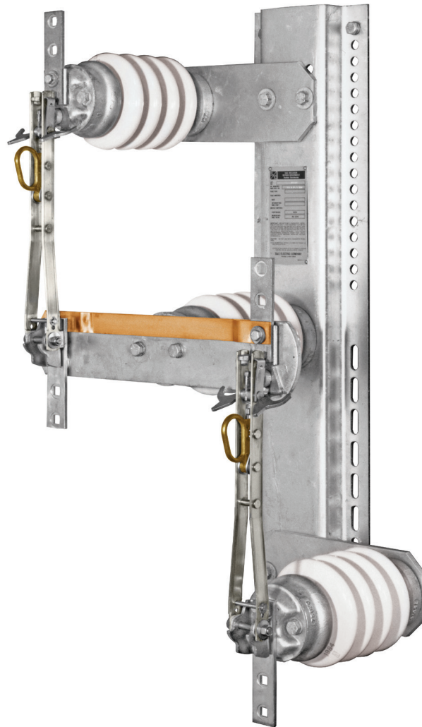
S&C Recloser Bypass Disconnect with Second Loadbuster Disconnect in Place of Fuse, furnished with porcelain station post insulators
