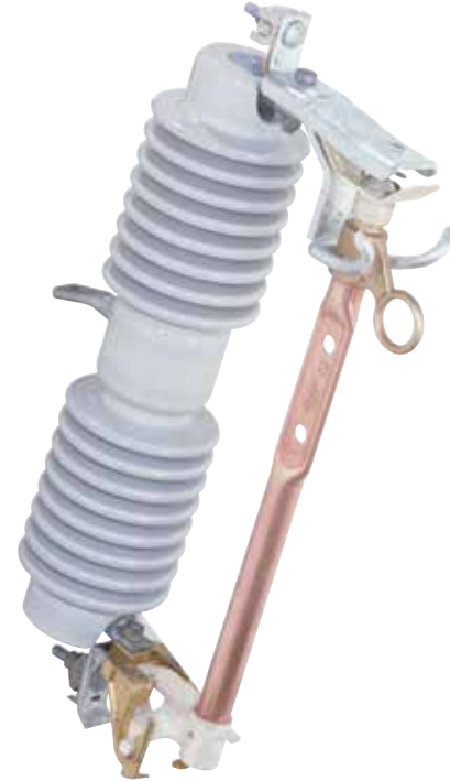
Catalog Number 89253R10-D▲ Disconnect, Overhead—Pole-Top Style, rated 25 kV nominal, 27 kV maximum, 150 kV BIL, 300 amperes continuous, 26 inches (660 mm) minimum leakage distance to ground.
