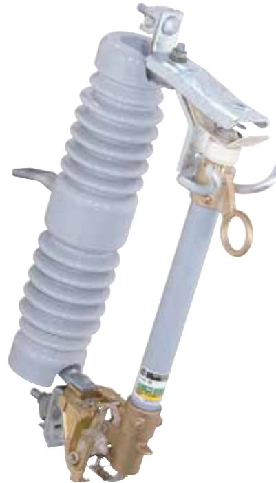
Catalog Number 89072R11-D▲ Ultra-Heavy-Duty Overhead—Pole-Top Style, rated 25 kV nominal, 27 kV maximum, 125 kV BIL, 200 amperes continuous, 10,000 amperes interrupting, RMS, asymmetrical, 11 inches (279 mm) minimum leakage distance to ground.
