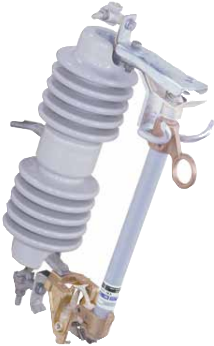
Catalog Number 89042R10-M★ Extra-Heavy-Duty Overhead—Pole-Top Style, rated 25 kV▼ nominal, 27 kV maximum, 150 kV BIL, 100 amperes continuous, 8,000 amperes interrupting, RMS, asymmetrical, 17 inches (432 mm) minimum leakage distance to ground.◆
