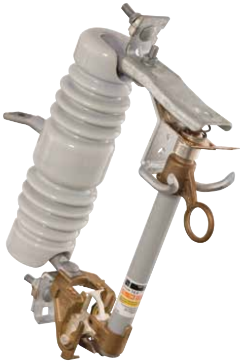
Catalog Number 89021R10-D▲ Extra-Heavy-Duty Overhead—Pole-Top Style, rated 14.4 kV nominal, 15 kV maximum, 110 kV BIL, 100 amperes continuous, 10,000 amperes interrupting, RMS, asymmetrical, 8½ inches (216 mm) minimum leakage distance to ground.
