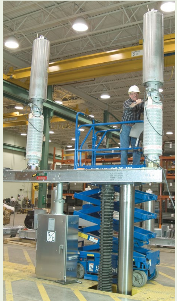
FIGURE 13. Each Series 2000 Circuit-Switcher is fully assembled, adjusted, and tested at the factory before shipment.
