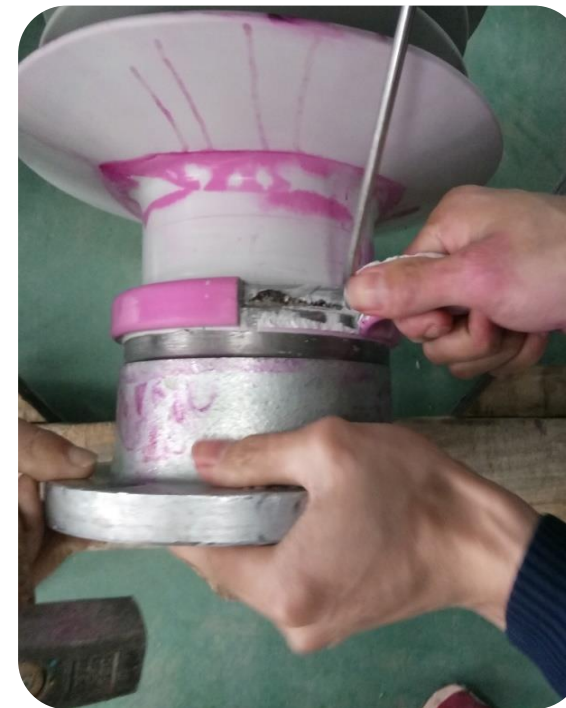
Penetration and Peeling Test 渗透和剥离试验
