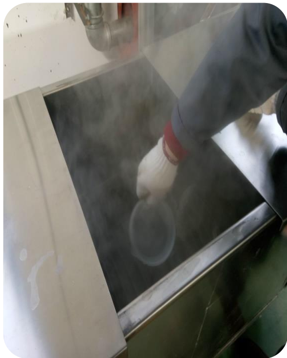
Water Immersion Pre-stressing Test 水煮试验
