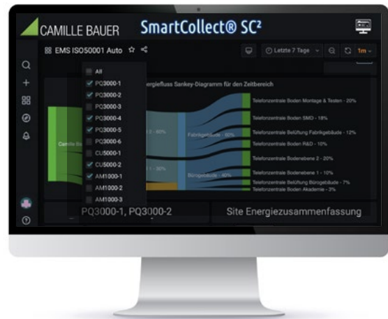
Graphics for individual measurement locations, incl. aggregation of measurement locations via time variable
