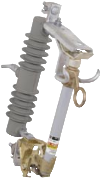
Catalog Number 89031R10-P-D▲ Ultra-Heavy-Duty Overhead—Pole-Top Style, rated 14.4 kV nominal, 15 kV maximum, 110 kV BIL, 100 amperes continuous, 16,000 amperes inter- rupting RMS asymmetrical, 8½ inches (216 mm) minimum leakage distance to ground.
