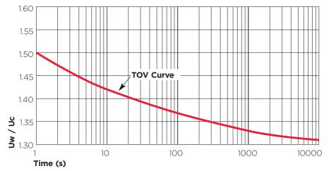
Temperature of samples (pre-heated): 60° C according to IEC 60099-4, Ed 2.0 2004. TOV Curve applies to an arrester which has a pre-stress applied prior to TOV verification. This pre-stress is equivalent to one high current impulse of 100kA, 4/10 as per the switching surge operating duty test.
