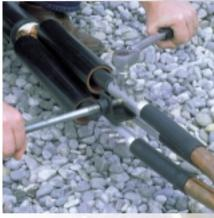
inside of the connector breaks up any conductor oxide layer and ensures reliable service over the entire life time of the joint. The connectors have been tested in accordance with IEC 61238-1 class A.
