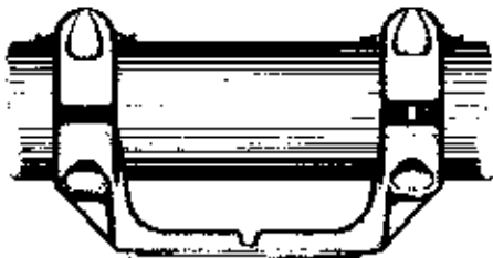
Tube support on insulator.
